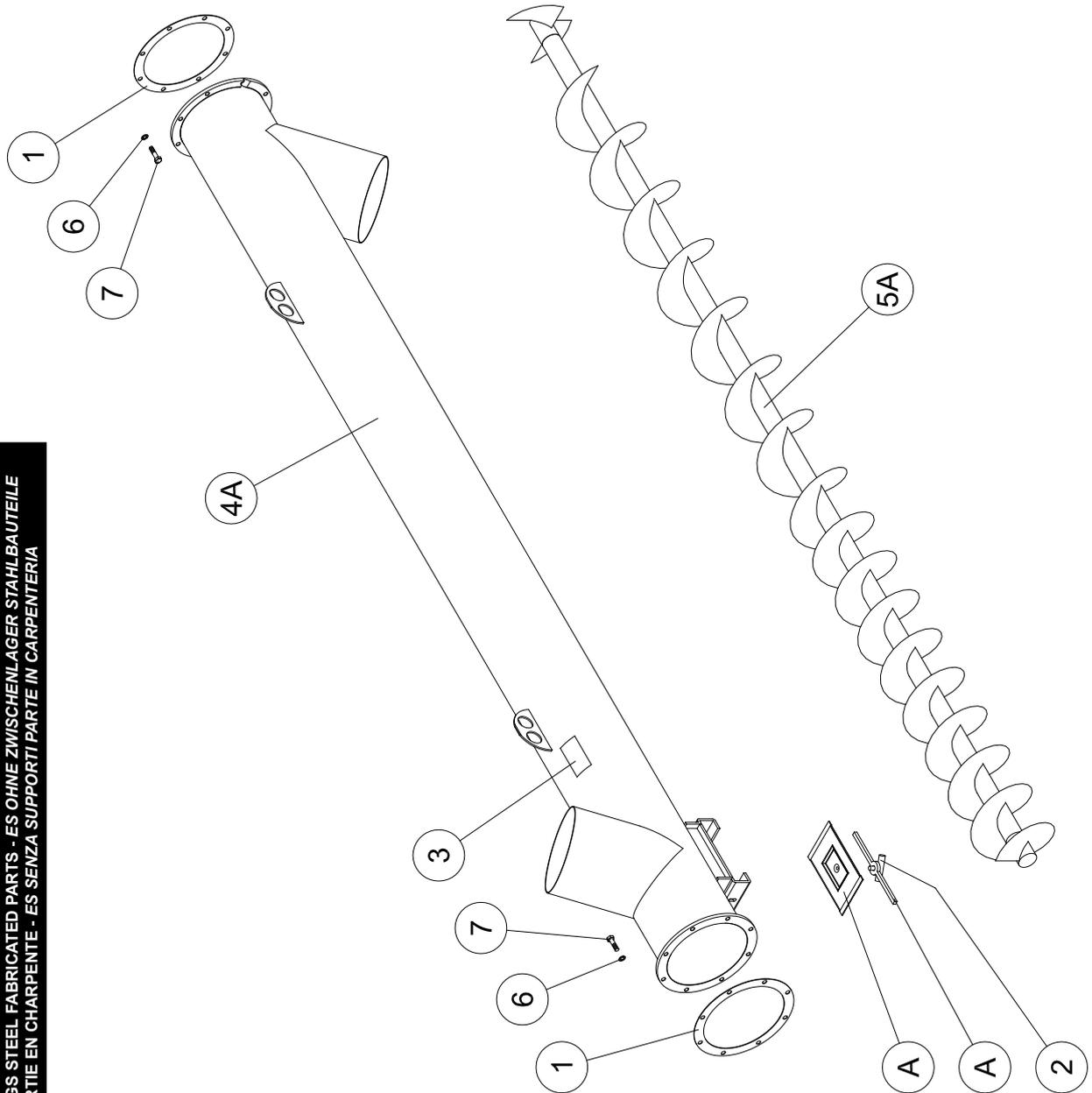
ES WITH ONE HANGER BEARING STEEL FABRICATED PARTS - ES MIT EINEM ZWISCHENLAGER STAHLBAUTEILE
